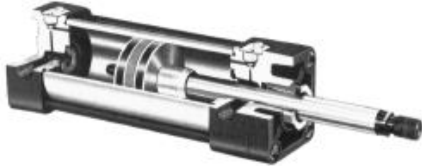
Figure 13-40. Construction of pneumatic cylinder. (Courtesy of Aro Corp., Bryan, Ohio.)
