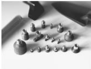
Figure 14-15. A variety of actual, different-sized vacuum cups. (Courtesy of Schmalz, Inc., Raleigh, North Carolina.)
