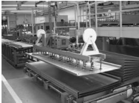
Figure 14-14. Factory application of the lifting and transporting of large sheet metal panels using pneumatic vacuum system technology. (Courtesy of Schmalz, Inc., Raleigh, North Carolina.)
