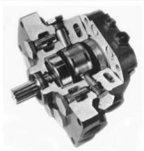
Figure 5-31. Cutaway view of a radial piston pump. (Courtesy of Deere & Co., Moltne, Illinots.)
