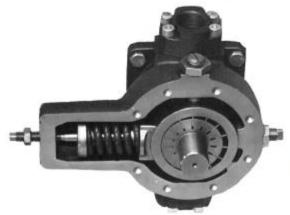
Figure 5-20. Cutaway photograph of pressure-compensated vane pump. (Courtesy of Continental Hydraulics, Division of Continental Machines, Inc., Savage, Minnesota.)
