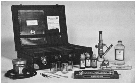
Figure 12-1. Hydraulic fluid test kit. (Courtesy of Gulf Oil Corp., Houston, Texas.)
