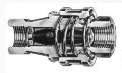
Figure 10-19. Quick disconnect coupling (cross-sectional view). (Courtesy of Hansen Manufacturing Co., Cleveland, Ohto.)
