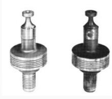
Figure 12-3. Corrosion caused by acid formation in the hydraulic oil. (Courtesy of Sperry Vickers, Sperry Rand Corp., Troy, Michigan.)
